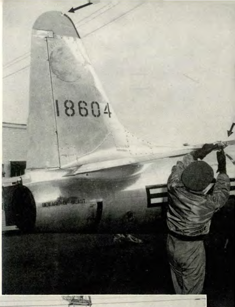
Pictured here are the large trees that sustained most of the impact. Right, damage to vertical and horizontal stabilizers clearly show that the aircraft flew below the trees tops. Note overall shot below.
